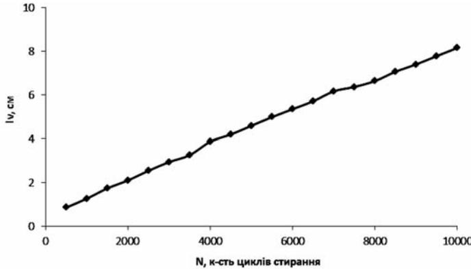
Fig. 2. The dependency of the volume wear of the photopolymer material on the number of friction cycles
