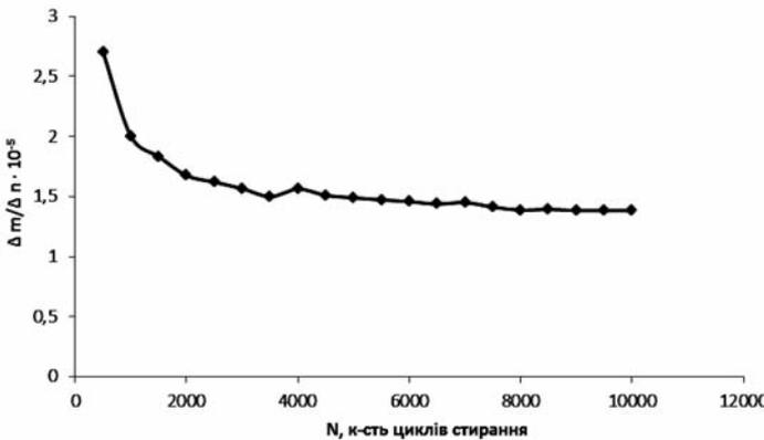
Fig. 3. The dependency of the gradient of the mass wear rate of the photopolymer material on the number of friction cycles
