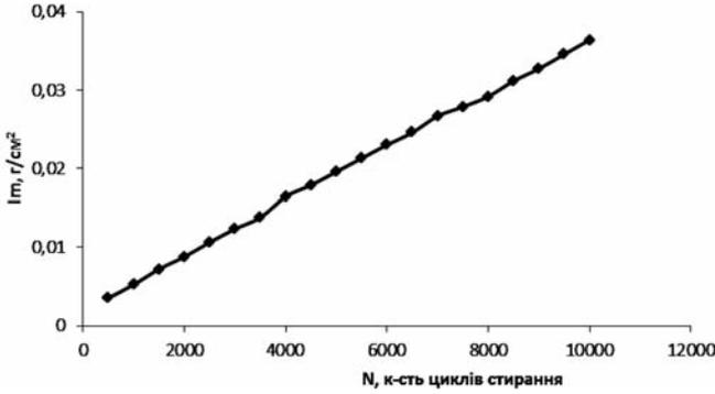
Fig. 1. The dependency of the specific wear of the photopolymer material (loss of mass) on the number of friction cycles
